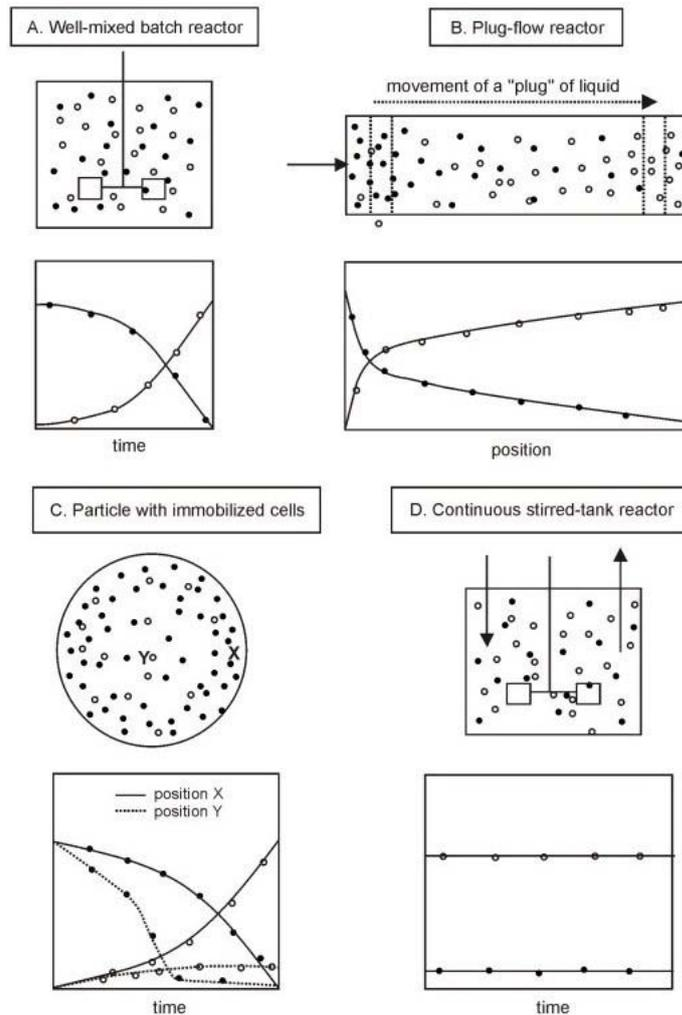
Figure 3: The influence of bioreactor operation on whether the state variables depend on position or time or both. On the graphs the vertical axis represents concentration. (●) Substrate (○) Product;
