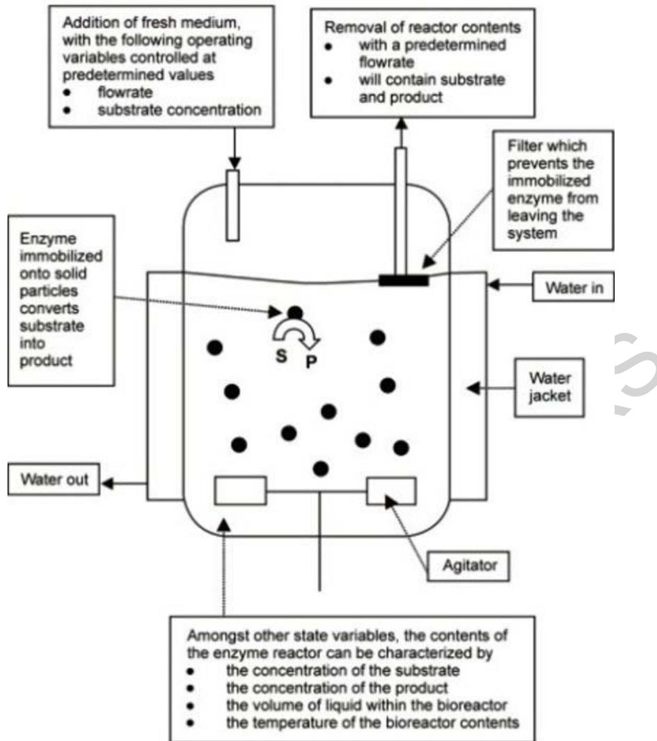
Figure 2: Diagram of an enzyme reactor, showing several of the important state and operating variables within the system
