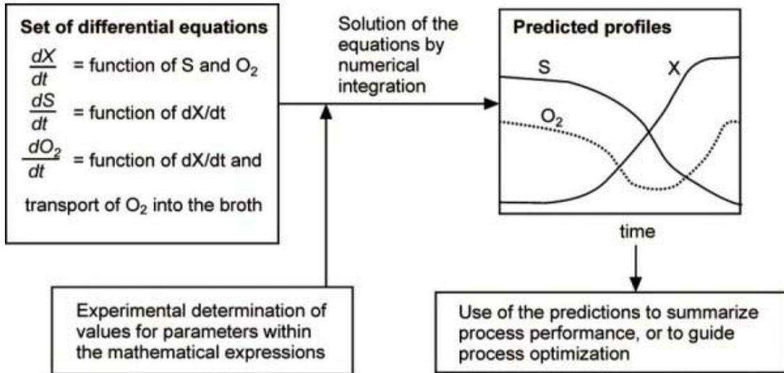
Figure 1: The application of a differential model to a fermentation process
