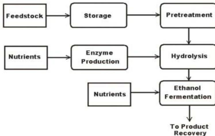
Figure 1a. Steps in a Biomass Refinery Using Enzymatic Hydrolysis
