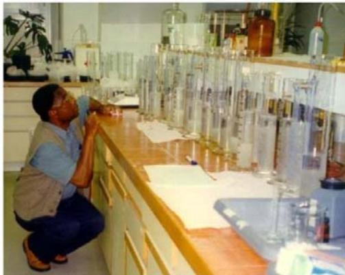
Figure 5: Testing superabsorbent water absorption properties (ICCS)
