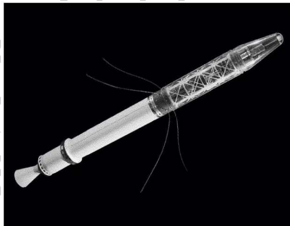
Figure 2. Explorer 1, the first US satellite, was launched on January 31, 1958. It's on orbit mass was 14 kg, not much compared to Sputnik 1's 84 kg. But Explorer 1 discovered the Earth's inner radiation belt, later called the inner Van Allen belt. (NASA)
