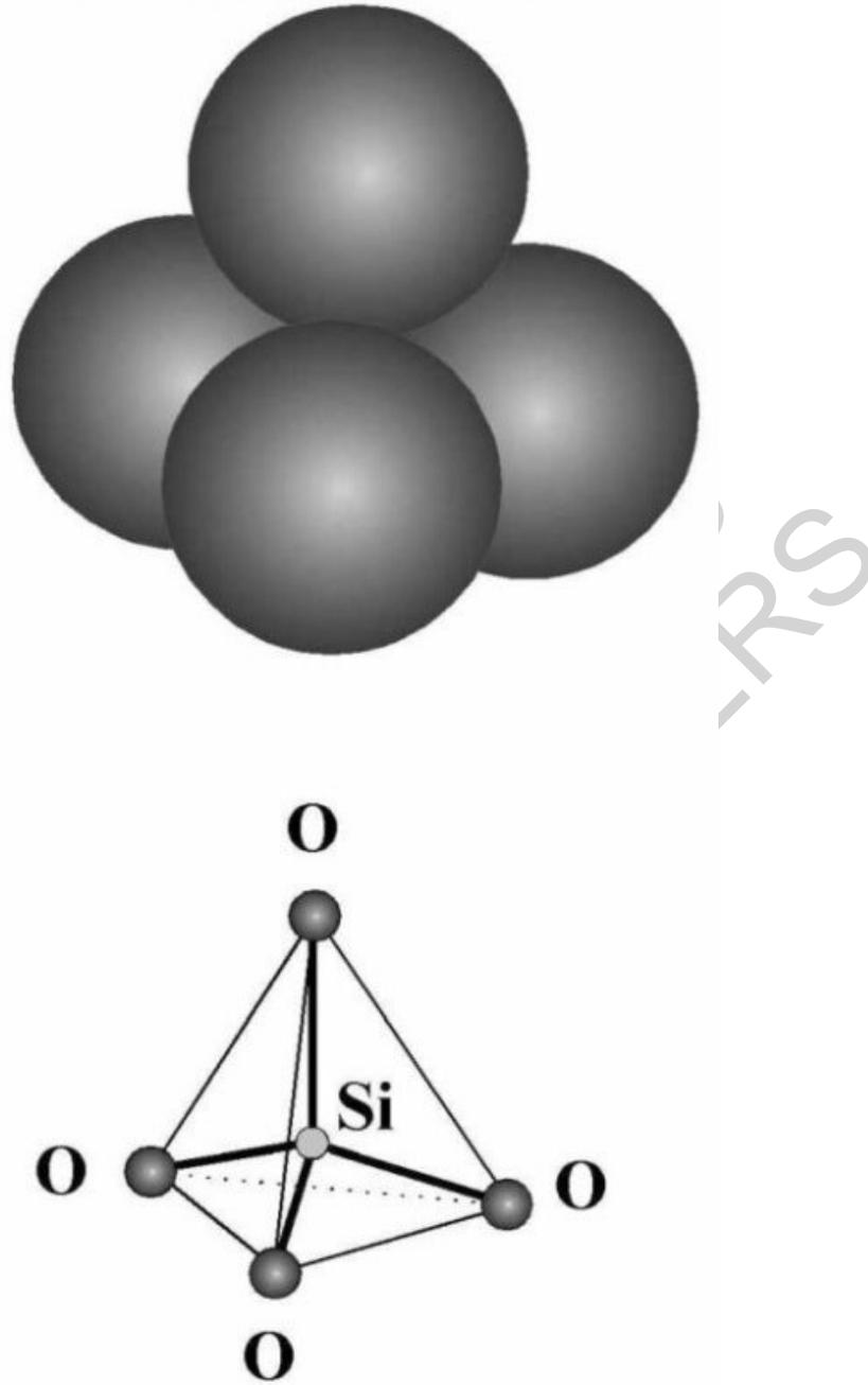
Figure 1. The  $\text{SiO}_4$  tetrahedron. The upper image shows an actual image of tetrahedron. Since oxygen ( $1.38 \text{ \AA}$ ) has a larger atomic radius than silicon ( $0.26 \text{ \AA}$ ), the silicon atom will completely disappear in the middle of the tetrahedron. The lower image shows a schematic ball-and-stick model of the  $\text{SiO}_4$  tetrahedron.
