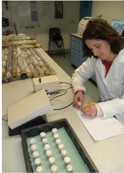
Figure 3. Using a Bartington MS2 magnetic susceptibility meter and MS2C dual frequency sensor.
