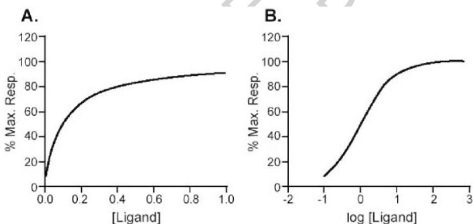
Figure 1: The Langmuir adsorption isotherm. A. Percent ligand bound (ordinates) as a function of the concentration of ligand according to Eq. (4). B. Semi-logarithmic version of the curve in panel A. The adsorption isotherm yields a characteristic sigmoidal curve with a logarithmic abscissa.
