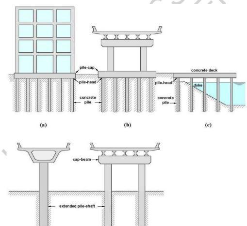
Figure 1. Various types of pile foundations: (a) group piles in a building foundation, (b) group piles in a bridge foundation, (c) group piles foundation in a wharf structure, (d) single-column bridge bent with extended pile-shaft, and (e) multi-column bridge bent with extended pile-shaft.
