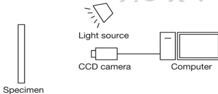
Figure 1 Setup for displacement measurement using digital image correlation
