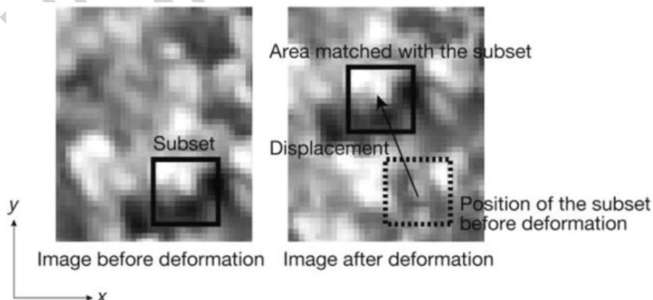
Figure 2 Matching the subset before and after deformation
