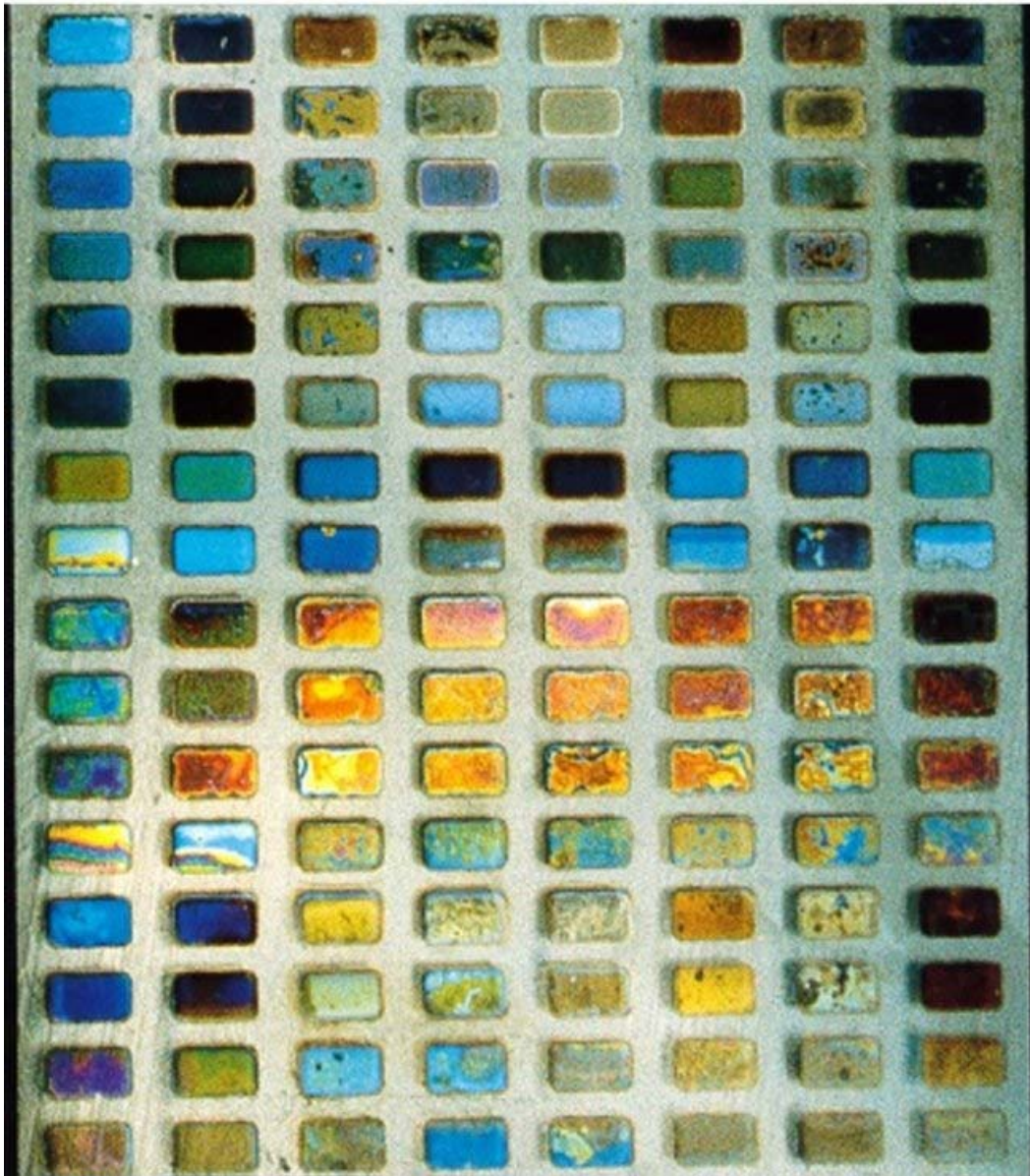
Figure 1. A Combinatorial Array (Library) of Ceramic Materials Prepared by Mixing Four Elements in Different Ratios. These are all potential superconductors, and each block will be tested individually to discover its properties
