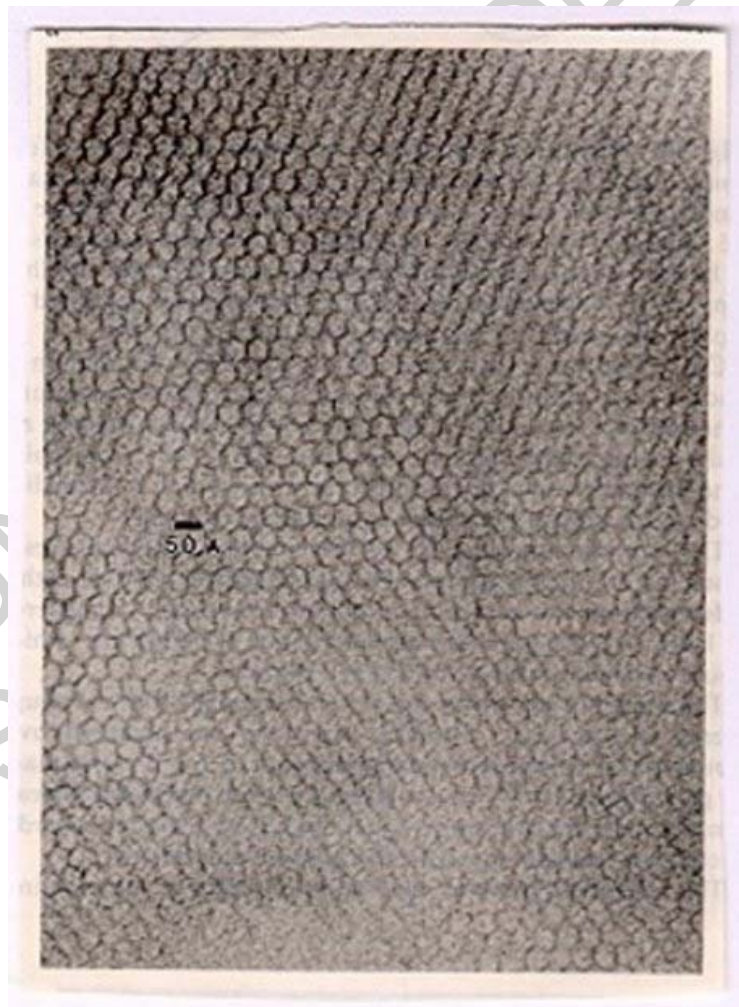
Figure 2. MCM-41, A Porous Form of Silica Permeated by Cylindrical Channels of Uniform Size. These can range from ~10–100 nm in width, depending on the method of preparation
