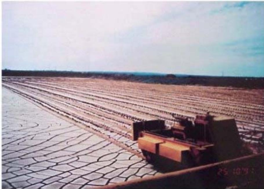
Figure 7. Alcoa Western Australia, bauxite waste dry stacking (Photograph courtesy of Alcoa of Australia)
