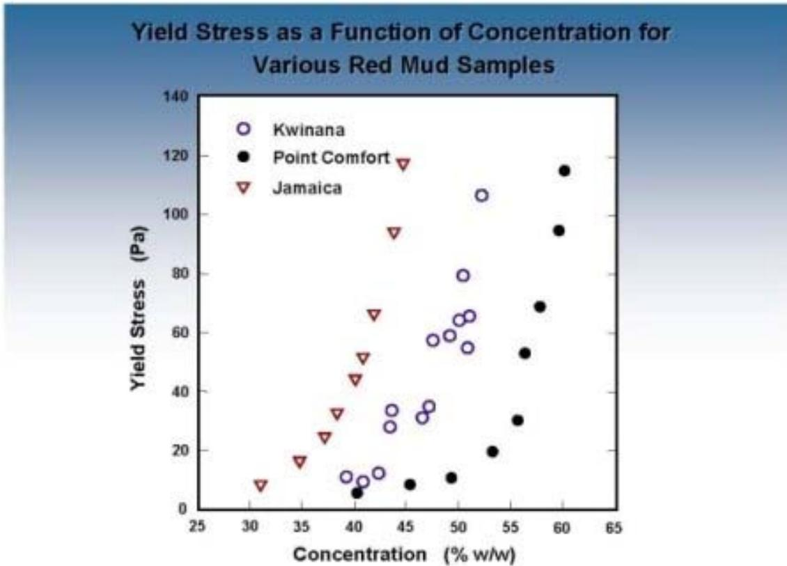
Figure 9. Yield stress as a function of concentration for red mud from different alumina samples
