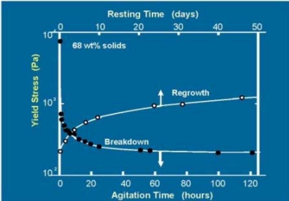
Figure 4. Use of the vane yield stress measurement to illustrate the breakdown and recovery of the red mud structure
