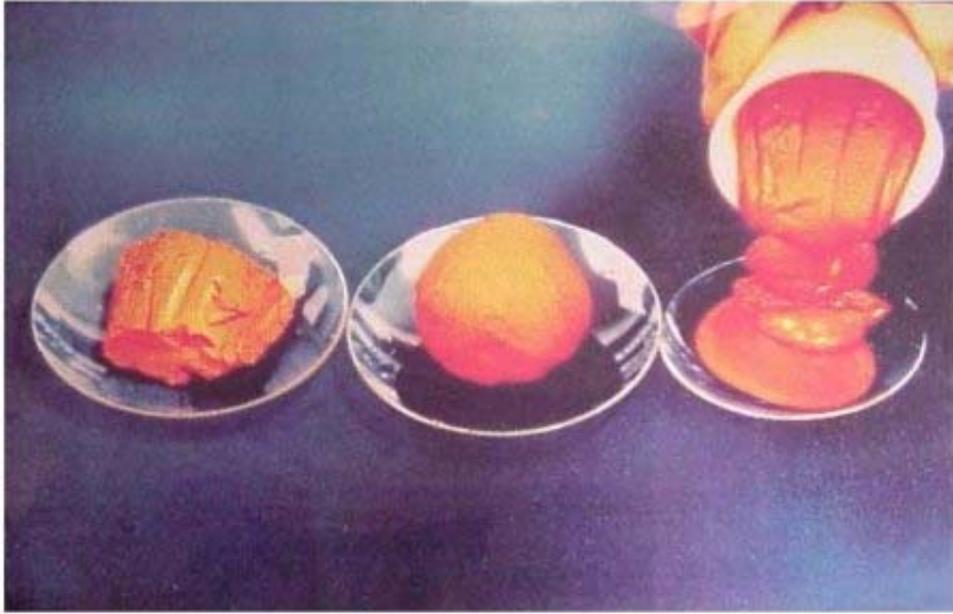
Figure 3. Illustration of the effect of shear on a red mud filter cake
