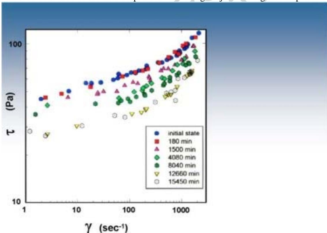
Figure 2. Typical red mud shear stress-shear rate behavior illustrating thixotropic behavior.
