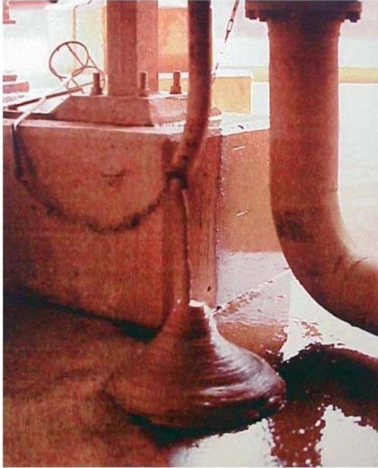
Figure 8. Mineral waste produced with a compression thickener (Photograph courtesy of Alcoa of Australia)
