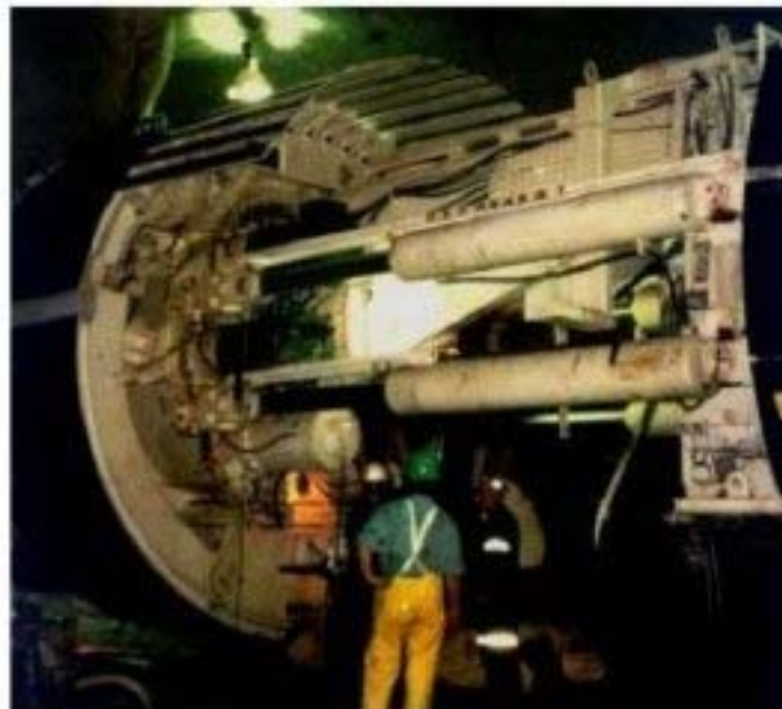
Figure 3: Typical side view of a tunnel boring machine. Courtesy of Harza Engineering Co., Chicago, IL, USA.
