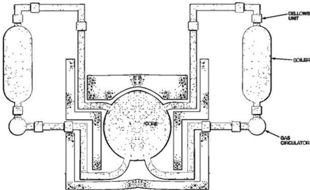
Figure 1: Magnox reactor steel pressure vessel and external boilers
