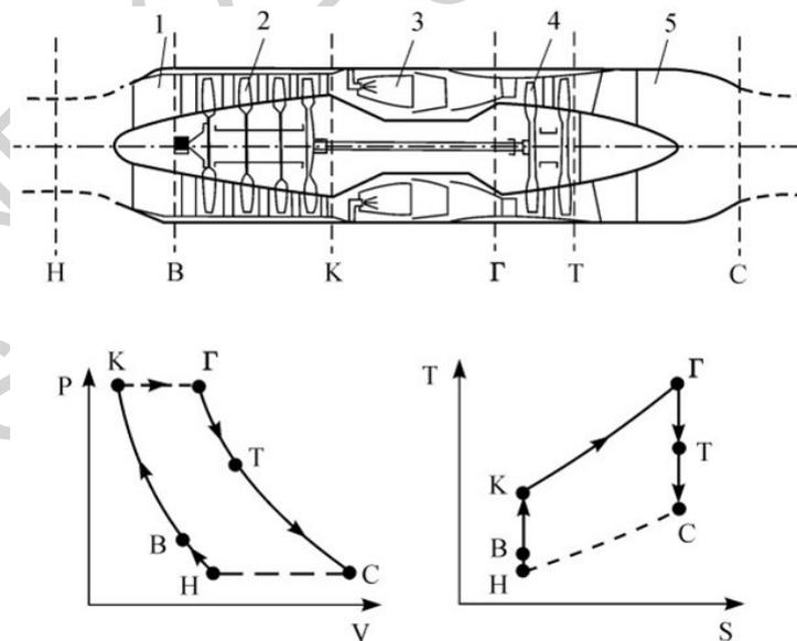
Figure1: Diagram of the turbojet and its thermodynamic cycle plotted in coordinates p-V and T-S. The dots show parameters in the cardinal cross section of the engine
