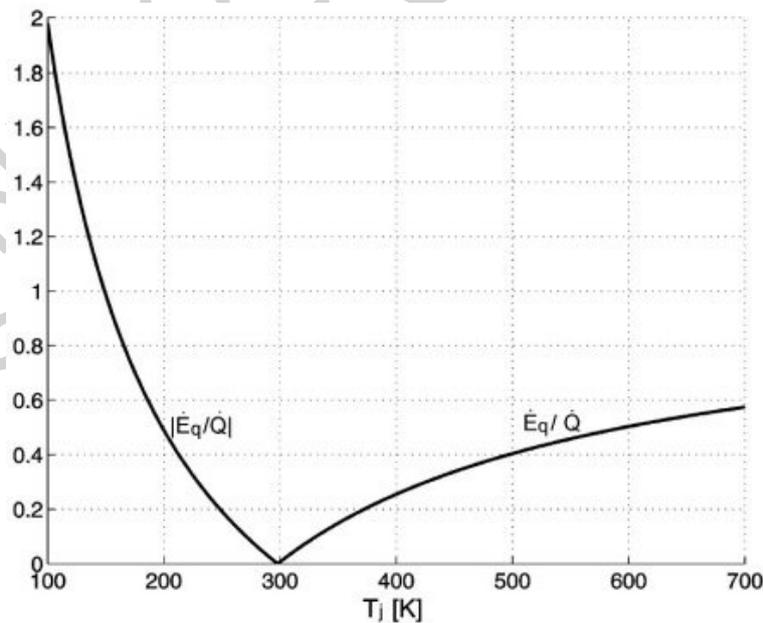
Figure 2: Exergy associated with the transfer of heat at different temperatures  $T_j$ . Here, the temperature of the environment is  $T_0 = 298.15K$ .
