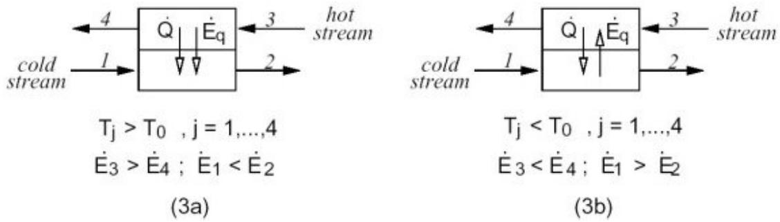
Figure 3: Heat exchangers operating above (Fig. 3a) and below (Fig. 3b) the temperature of the reference environment  $T_0$ .
