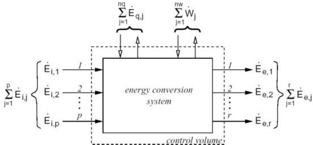
Figure 1: Schematic diagram to illustrate the exergy balance for a control volume system.
