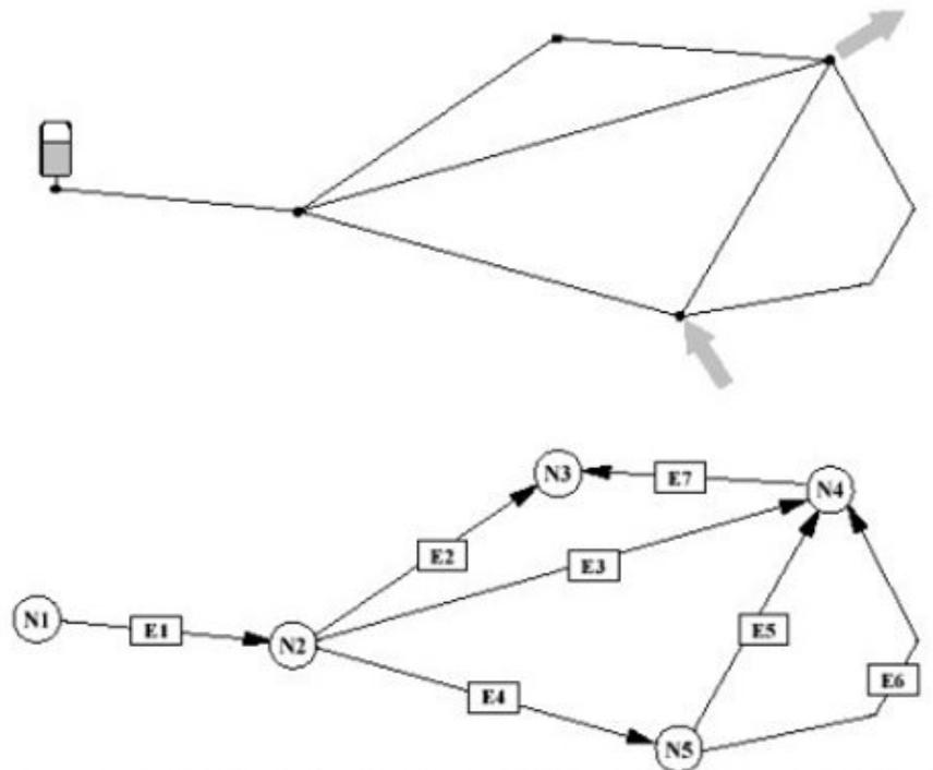
Figure 3. A simple pipe network with one reservoir at constant pressure, one inflow and one outflow (in gray)
