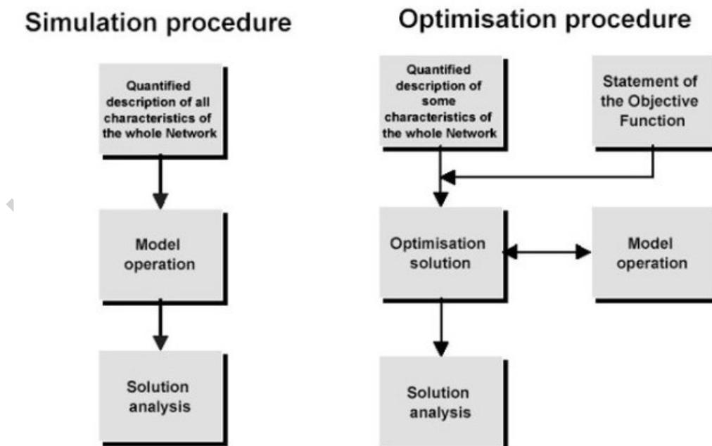
Figure 1. Schemes of the solution procedures
