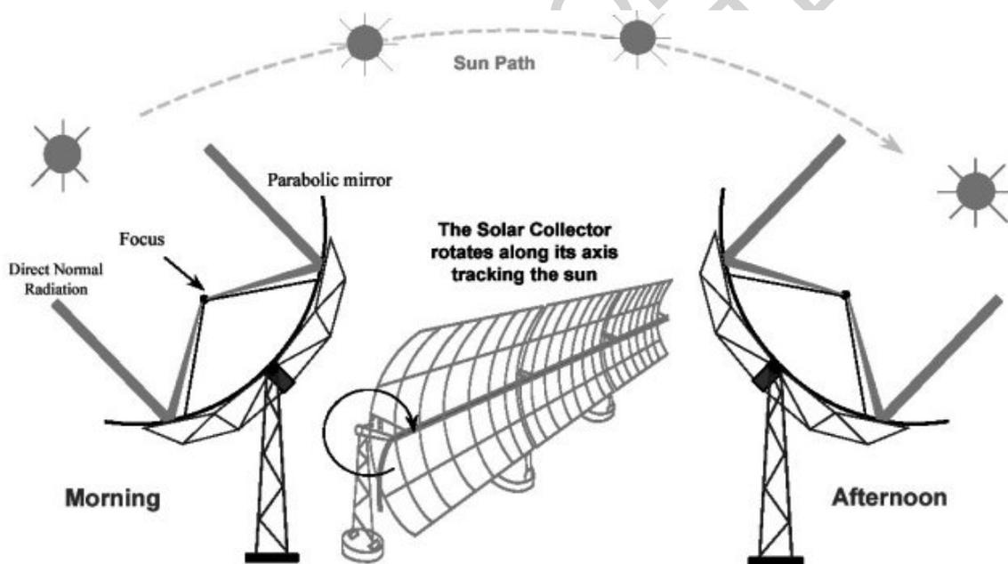
Figure 3. Solar ray reflection on a one-axis parabolic trough collector
