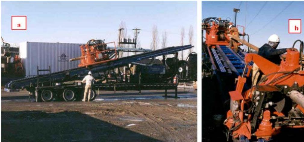
Figure 3. Trailer-mounted HDD Maxi Rig - 500,000 lbf (2200 kN) Capacity; (a) As-mobilized rig prior to set up; and (b) Drill rod being added during operation.
