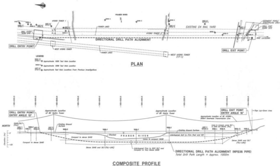
Figure 1. Example of a below-water pipeline river crossing; plan and profile of design pipeline alignment– Terasen Gas Fraser River Crossing Project, Coquitlam/Surrey, B.C.
