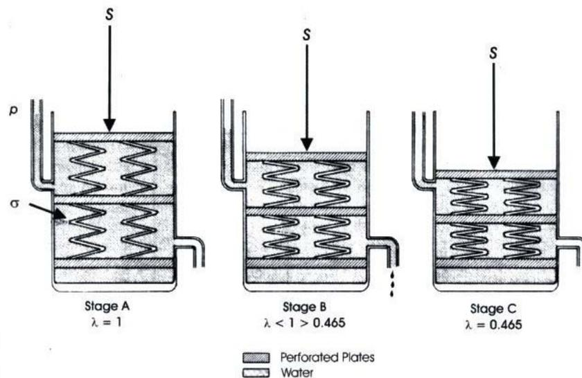
Figure 1. Schematic representation of compaction.  $\sigma$  = grain-to-grain strength.  $S$  = axial component of total stress (overburden pressure), and  $p$  = fluid pressure,  $\sigma = S - p$ . Stage A) initial pressure system. Stage B) some water is allowed to escape; springs now carry a greater part of applied load. Stage C) compaction equilibrium; load is supported jointly by springs and the water pressure, which is hydrostatic.
