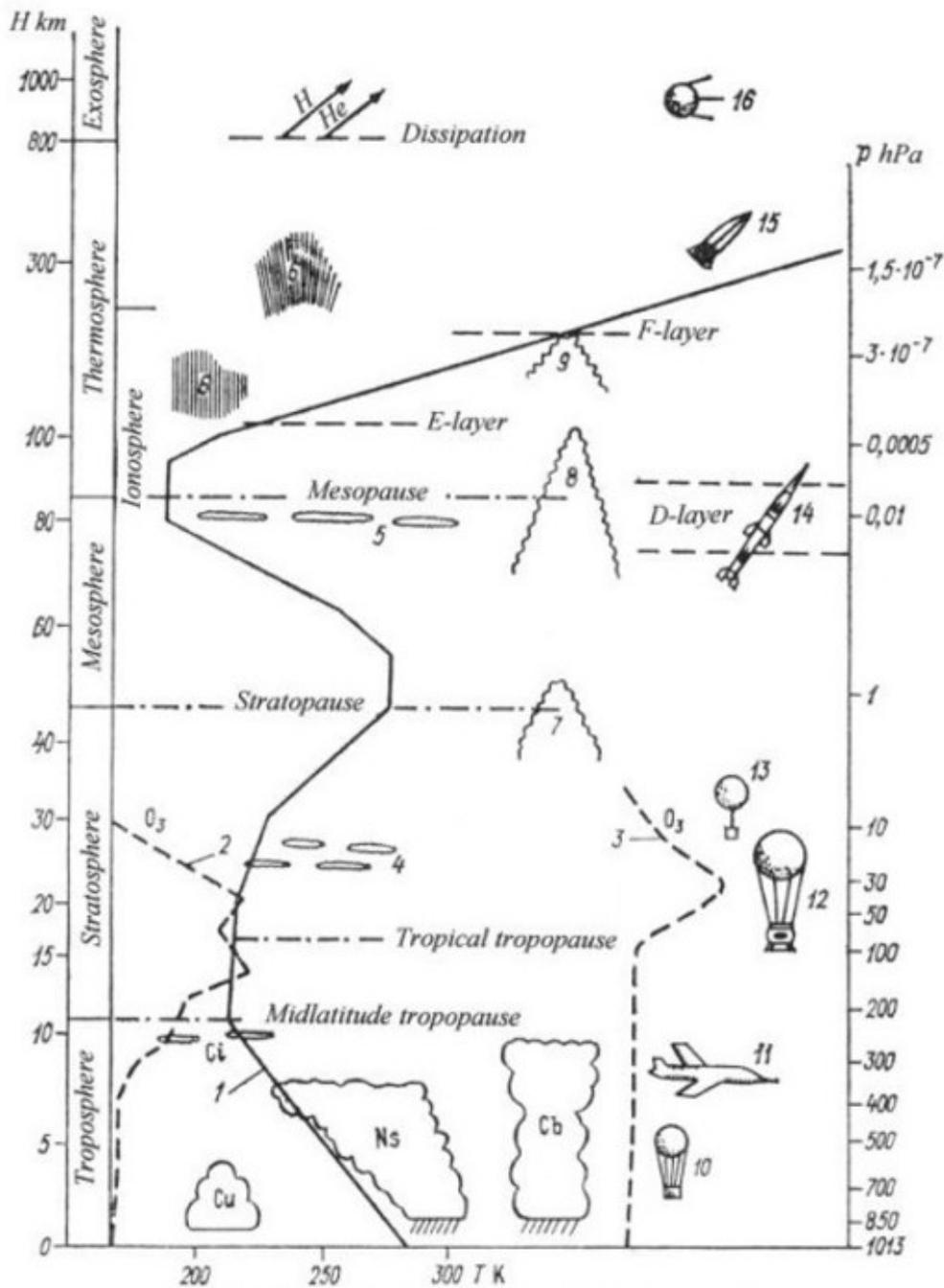
Figure 1. Structure of the atmosphere and methods of investigation
