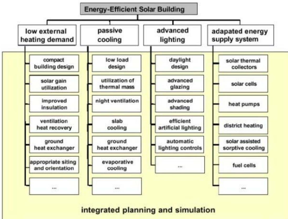
Figure 1: Main Components of solar buildings (C.F. Reinhart et al. 2001)
