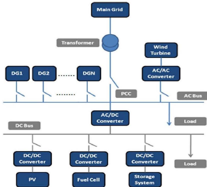
Figure 1. Schematic diagram of a microgrid
