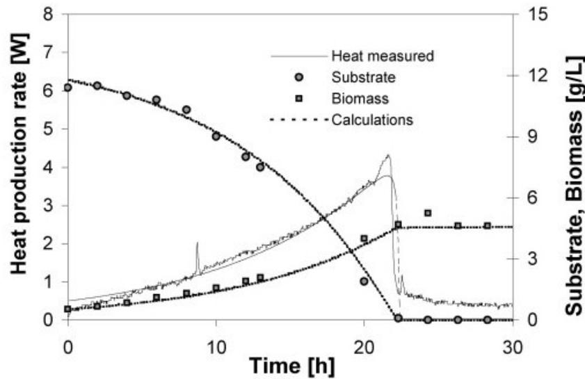
Figure 2: Test of the bioreactor used as an “off the peg” calorimeter. Comparison of the calculated with the measured heat production rate for the aerobic growth of *H. elongata* on glycerol.
