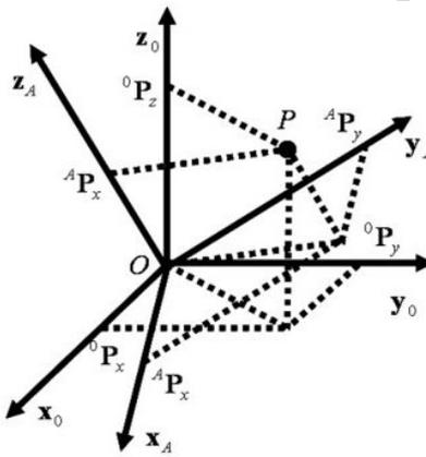
Figure 6: Representation of a point  $P$  in two different coordinate frames.
