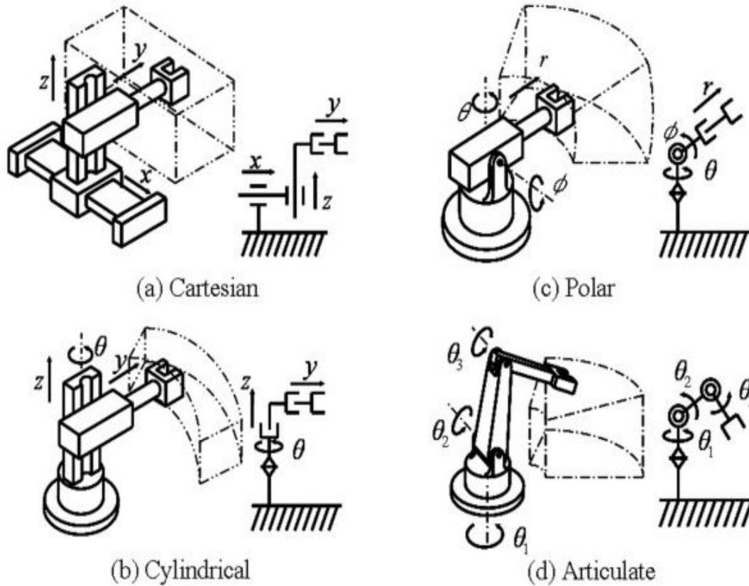
Figure 3: Robot configurations
