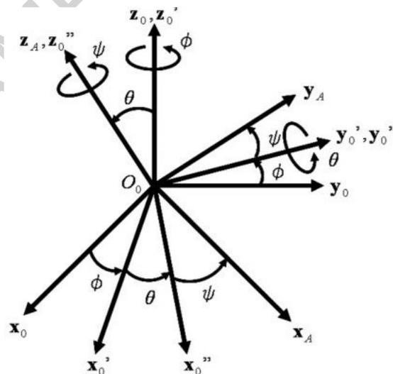
Figure 7: Representation of Z-Y-Z Euler angles.
