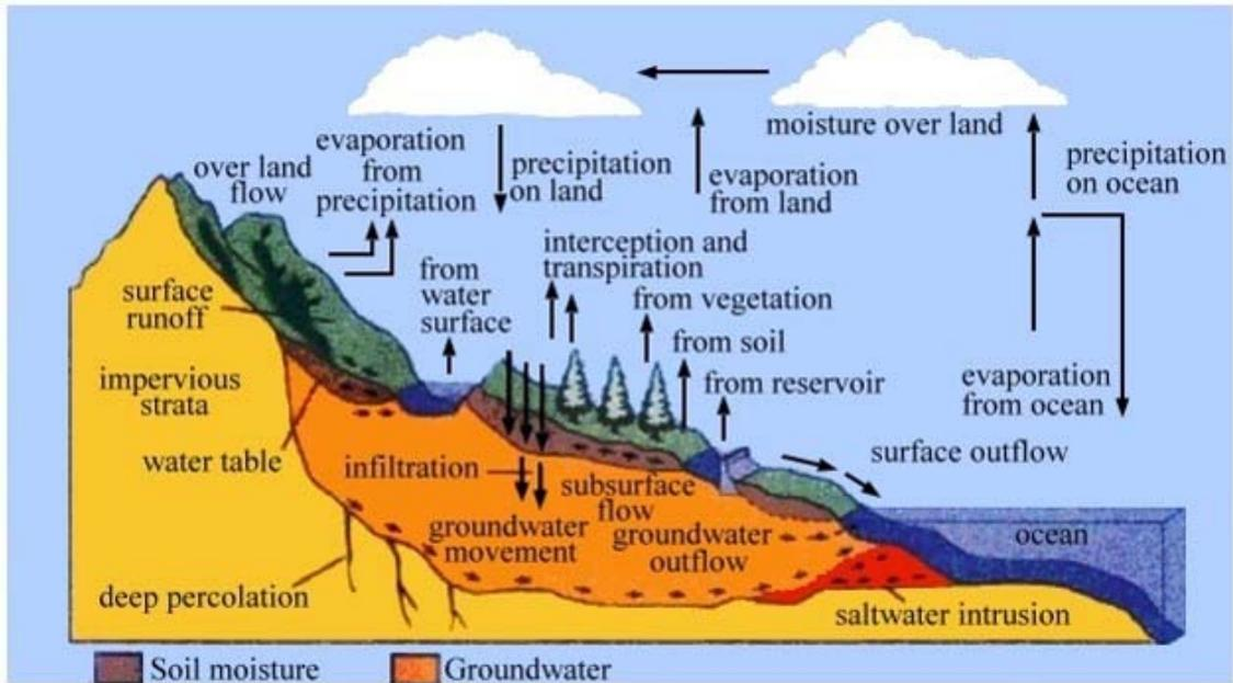
Figure 3. Hydrological cycle.
