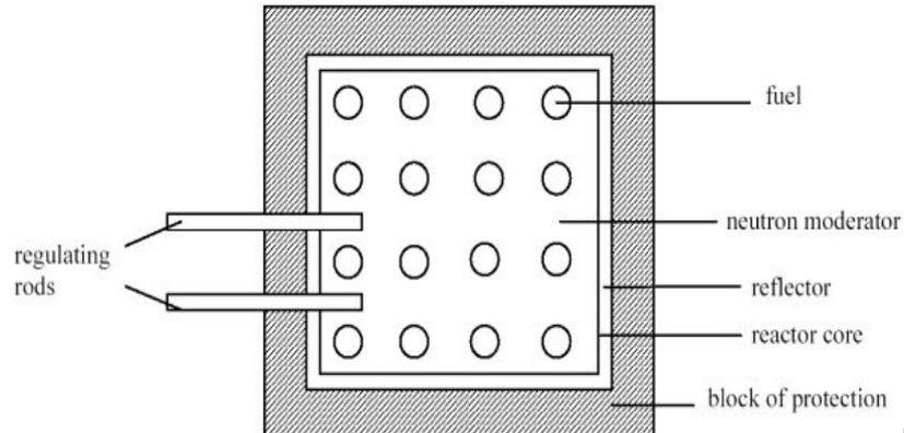
Figure.1 – Simplified scheme of reactor's section.
