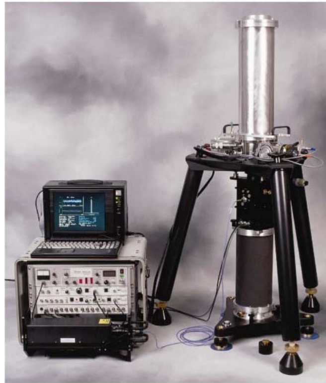
Figure 2: Principle of the FG5 absolute gravimeter
