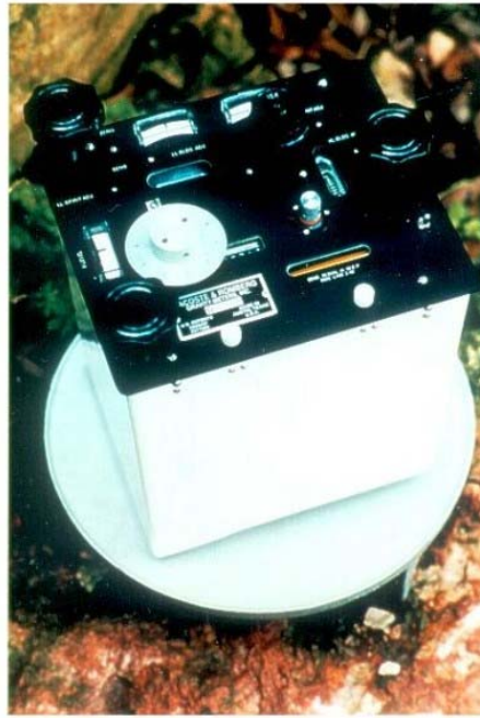
Figure 7. Photography of a LaCoste Romberg gravimeter
