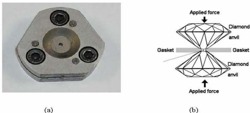
Figure 6. (a) A view of a diamond anvil cell (DAC) for high pressure crystallography; (b) a schematic view of a DAC. The sample compartment (arrowed) contains hydrostatic fluid, the sample and a small ruby for measuring the pressure.
