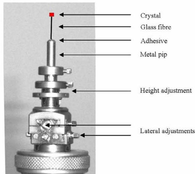
Figure 2. A red crystal mounted on a glass fiber. The fiber is glued to a metal pip which fits into the well of a goniometer head, ready for mounting on a diffractometer.
