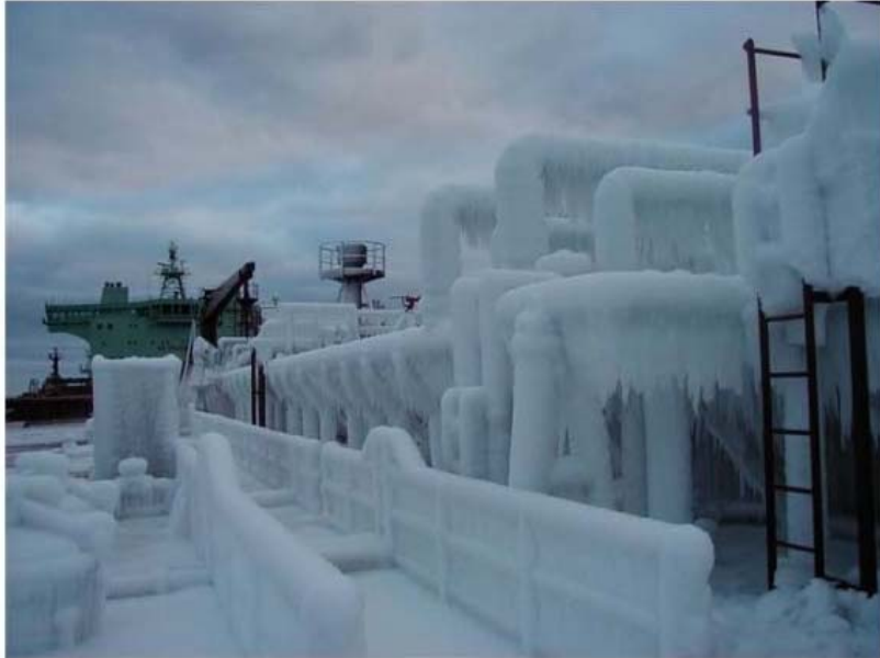
Figure 6. Icing on the deck of a tanker (photo Mari Hoikkala).
