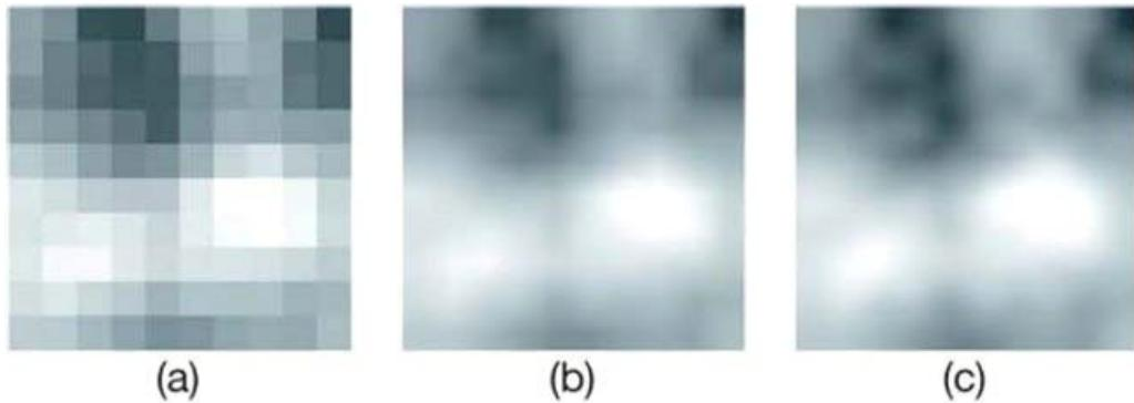
Figure 5 (a)  $10 \times 10$  pixels region; (b) bilinear interpolation; (c) bicubic interpolation
