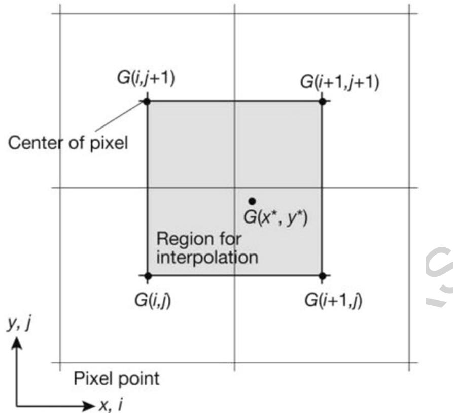
Figure 4 Pixel points and interpolating region for bilinear interpolation
