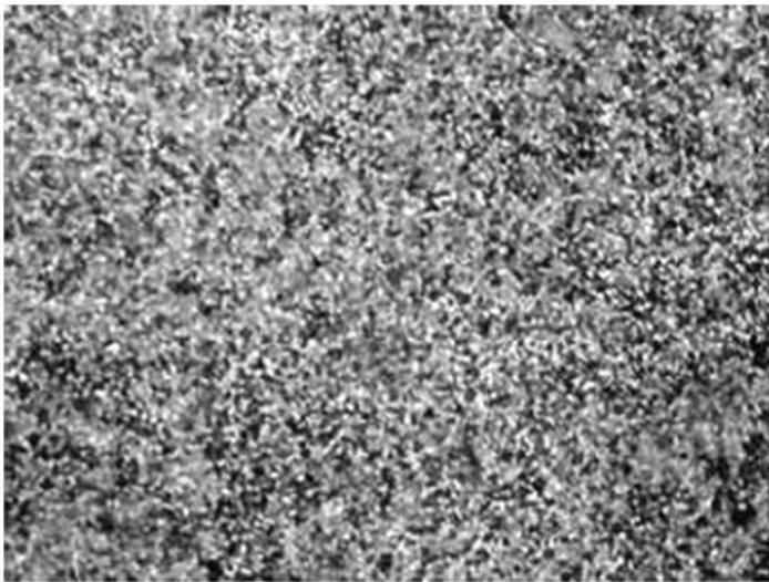
Figure 3 Typical example of random pattern on specimen surface
