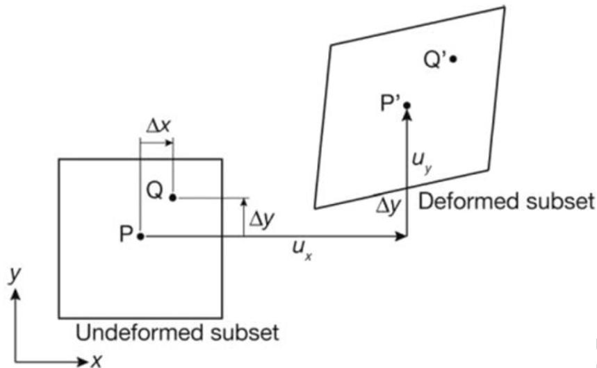
Figure 6 Subset before and after deformation
