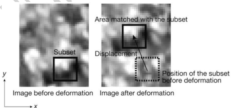
Figure 2 Matching the subset before and after deformation
