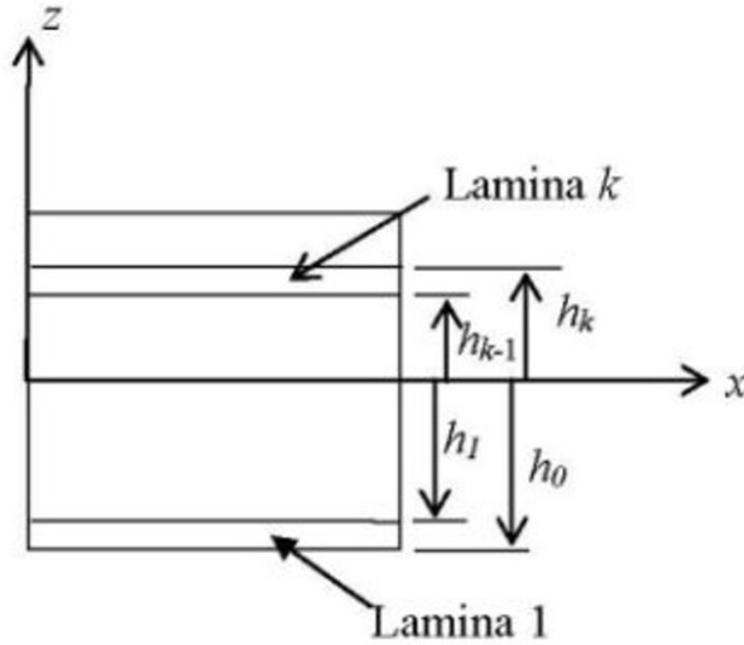
Figure 3. Laminate with coordinate notation for individual lamina
