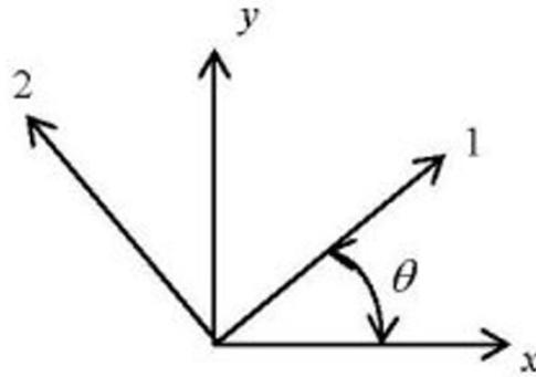
Figure 1. Coordinate system for transformation between the principal material axes and the x-y coordinate system
