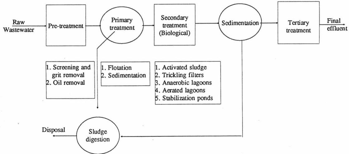
Figure 2. Schematic Flow Diagram of a Typical Wastewater Treatment
