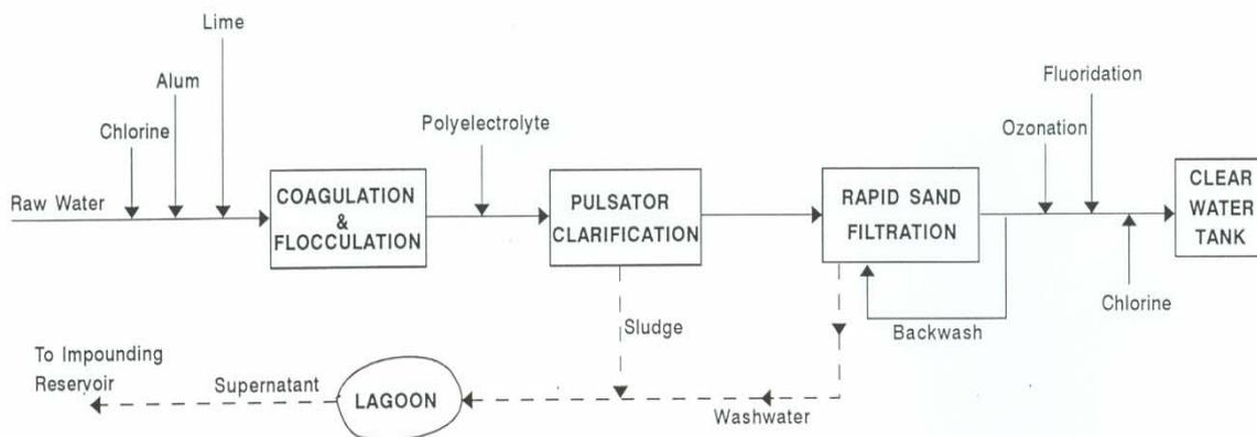
Figure 1. Schematic Unit Processes in a Typical Water Treatment Plant
