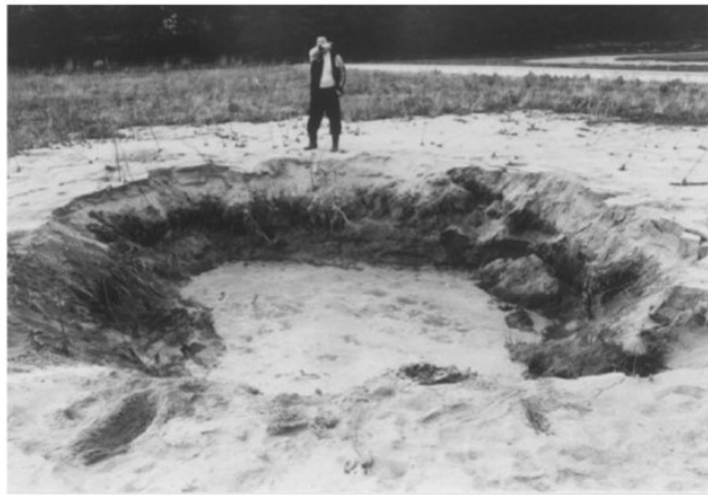
Figure 7. Ground Inundated with Spouting Sand (Taken by H. Takeuchi)
