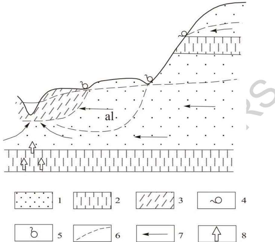
Figure 3. Scheme of groundwater discharge into a river valley
