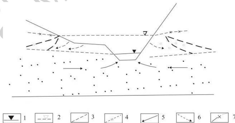
Figure 2. Scheme of interaction between surface and ground water under hydraulic relations (in permeable strata)
