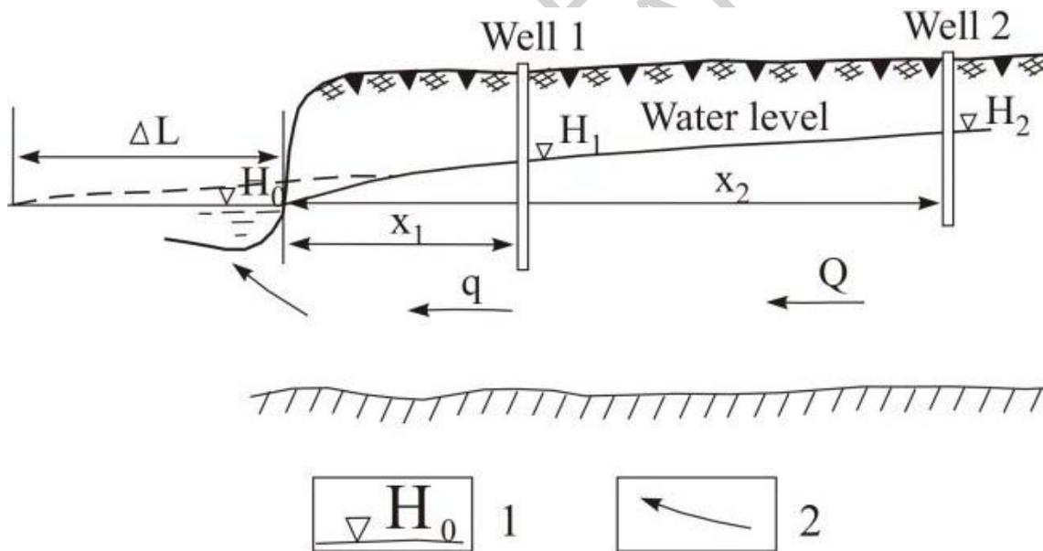
Figure 4. Scheme of assessing the river bed resistance ( $\Delta L$ ) to the levels of surface and ground water
