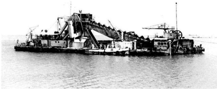
Figure 8. Modern diesel-electric driven bucket dredger
