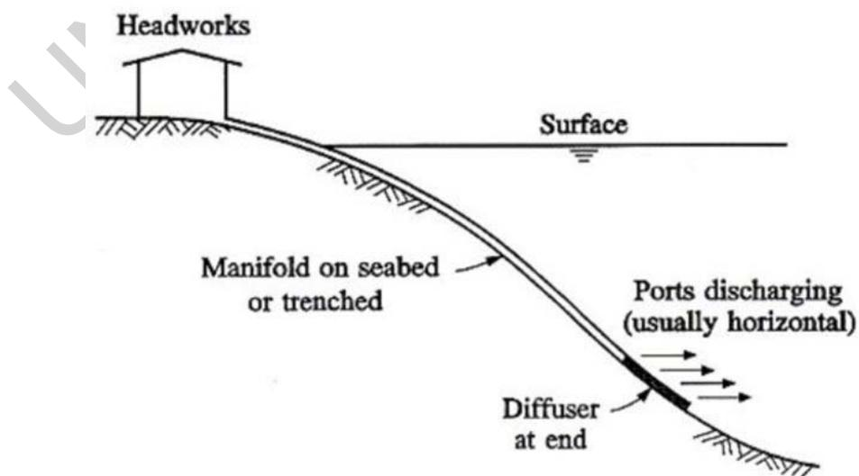
Figure 1. Typical arrangement for small outfall
