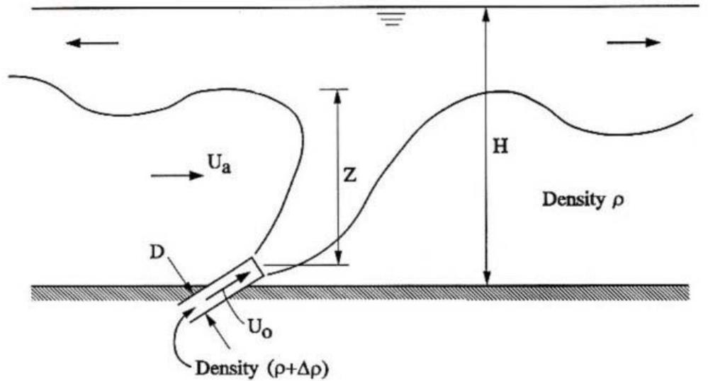
Figure 3. Submerged buoyant jet discharging into water of finite depth
