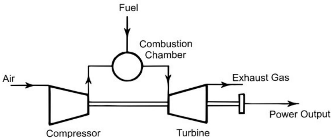
Figure 1. Simple gas turbine system
