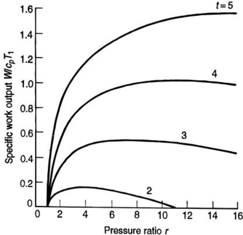
Figure 5. Specific work output for simple cycle
