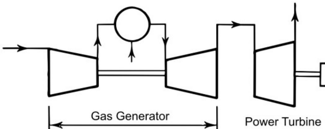
Figure 2. Gas turbine with separate power turbine
