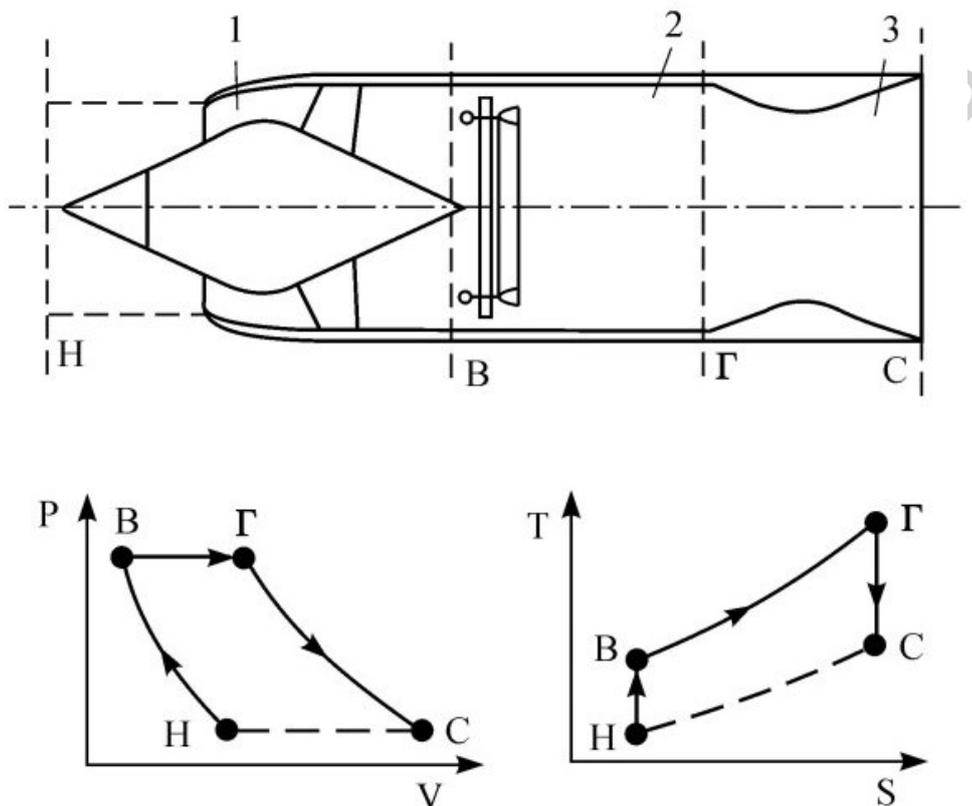
Figure 3: Diagram of the scramjet and its cycle in coordinates  $p$ - $V$  and  $T$ - $S$ .
