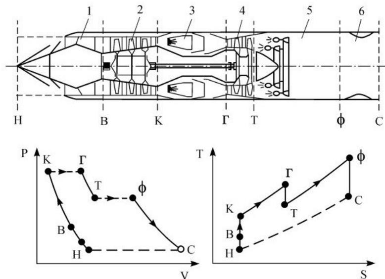
Figure 2: Diagram of the turbojet with afterburner and its thermodynamic cycle in coordinates  $p$ - $V$
