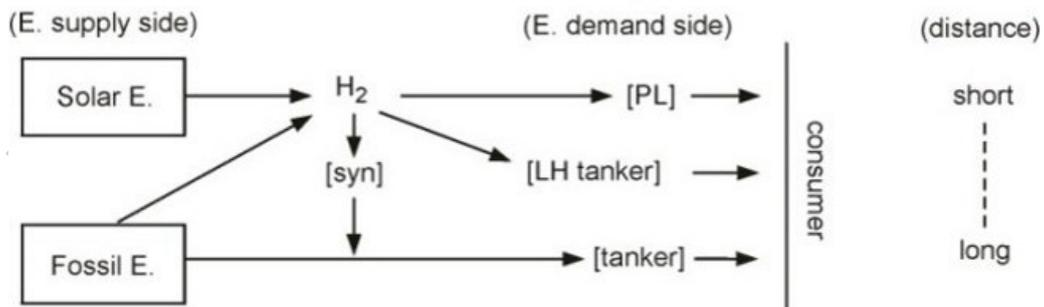
Figure 2. Position of liquid hydrogen tanker system; E: energy, syn: synthesis, PL: gas pipe line, LH: liquid hydrogen
