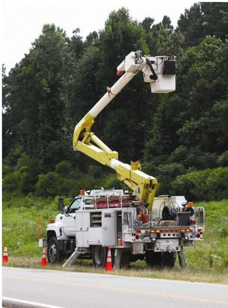
Figure 2. Mobile Elevated Working Platform © NEBOSH
