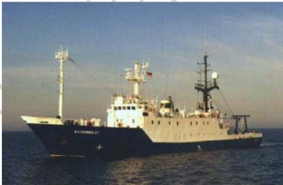
Figure 1. Research vessel (r/v) Alexander von Humboldt of the Institute for Baltic Sea Research Warnemuende (IOW), Germany. Launching: February 1967; completion: July 1967; length: 64.23 m; gross tons: 1270.58; range: long distances; total rated power: 1750 hp; speed: 12 knots; labs: 7 + CTD laboratory; crew: 15; scientists 13.
