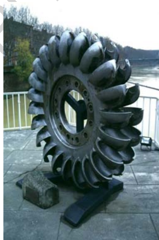
Figure 2. Turbine, Pelton Wheel, Bazacle hydro-electric power plant (Toulouse, France).
