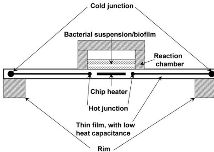
Figure 1: Measurement principle of a chip calorimeter.
