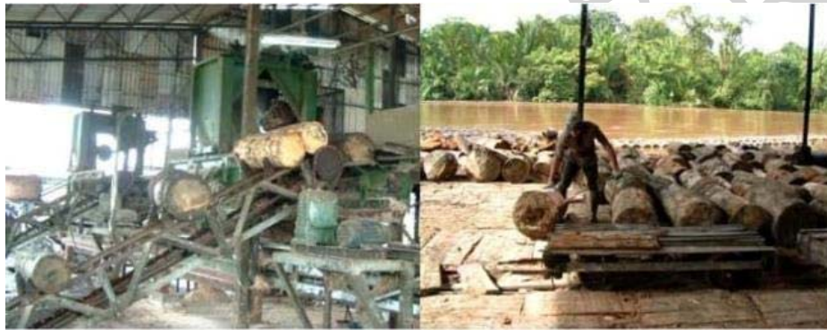
Figure 4: Sago logs are debarked using either an auto debarking machine or manually with a machete.
