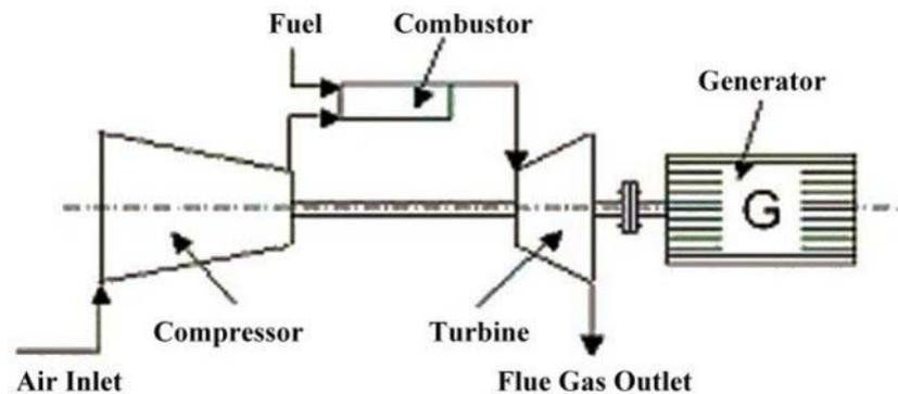
Figure1: Single shaft power block.
