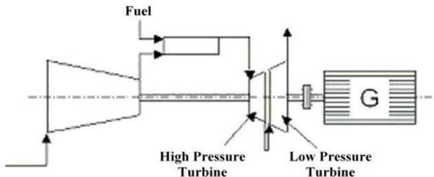
Figure 2: Two shaft, single cycle power block.
