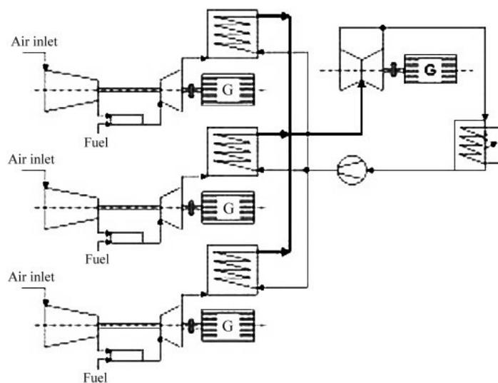
Figure 5: Multi shaft, combined cycle power plant setup.
