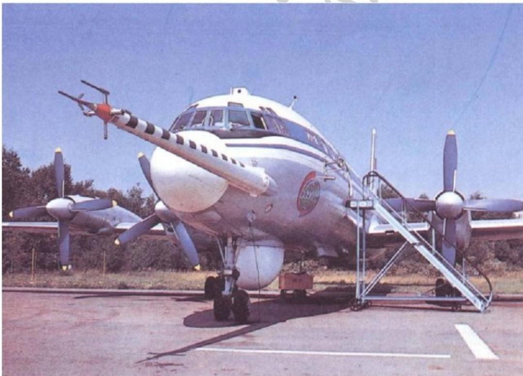
Figure 1: Flying laboratory “Ilyushin-18” equipped with different sensors for measurements of atmospheric parameters and tools for cloud seeding. It was used in various research and operational projects for weather modification
