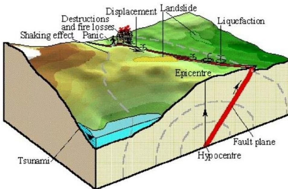
Figure 1. Earthquake source and its secondary effects
