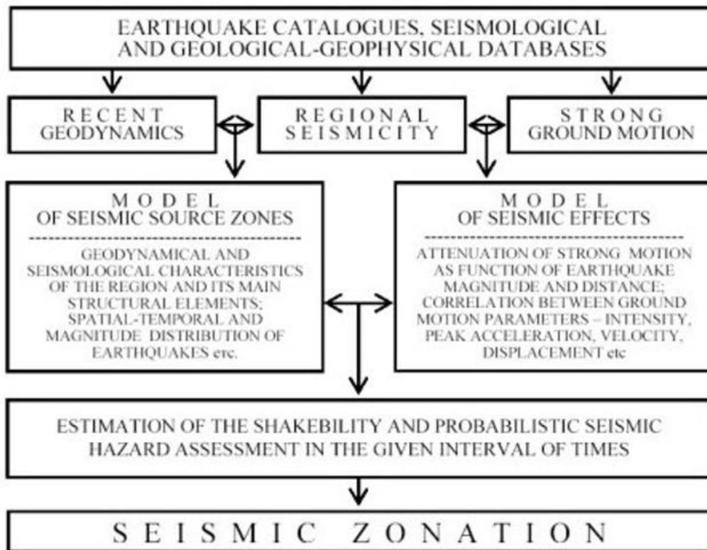
Figure 2. Structural chart of seismic zoning methodology.
