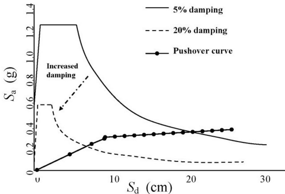
Figure 1. Capacity spectrum procedure to determine performance point of the structure.
