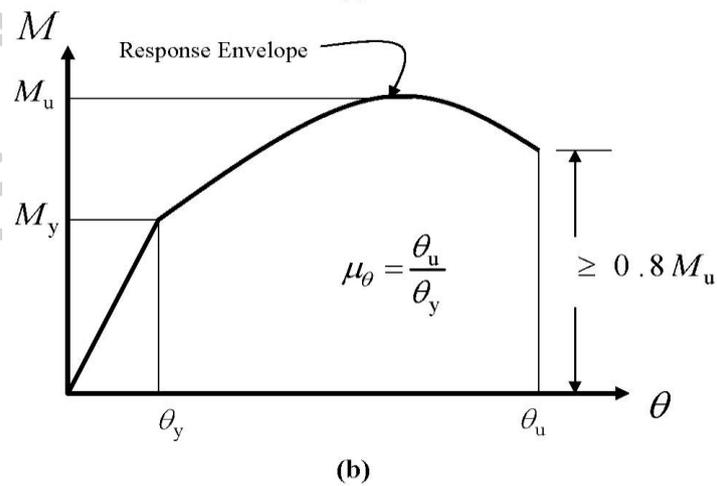
Figure 1. Load-Deformation Curves
