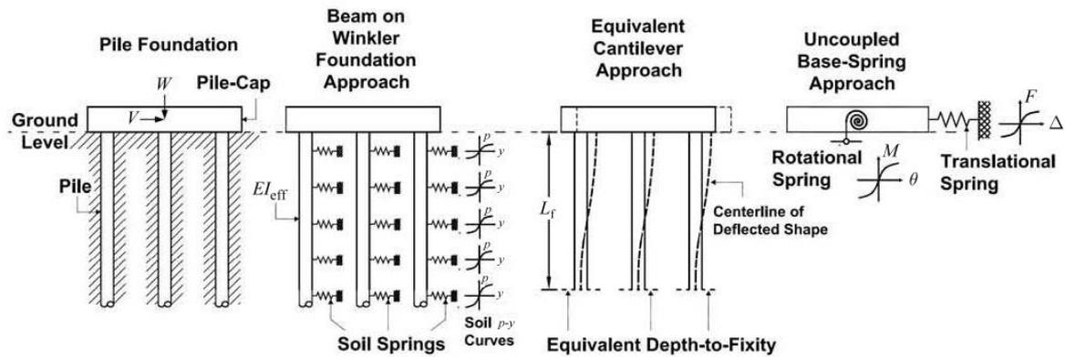
Figure 3. Various approaches for modeling laterally loaded pile foundations
