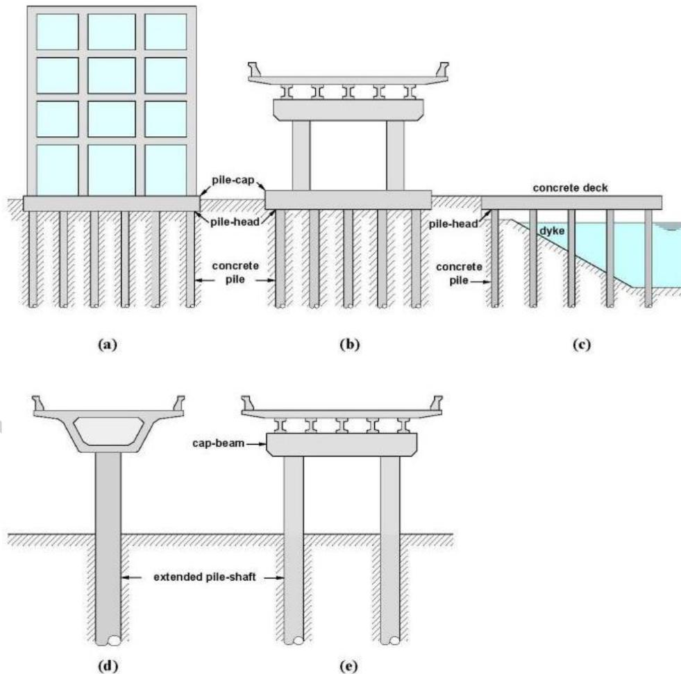
Figure 1. Various types of pile foundations: (a) group piles in a building foundation, (b) group piles in a bridge foundation, (c) group piles foundation in a wharf structure, (d) single-column bridge bent with extended pile-shaft, and (e) multi-column bridge bent with extended pile-shaft.
